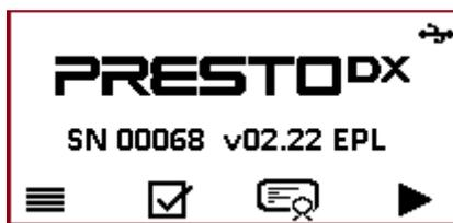
The bottom line will advise you with proper icons about available functions. Press the device key below the icon to execute the proper function.
